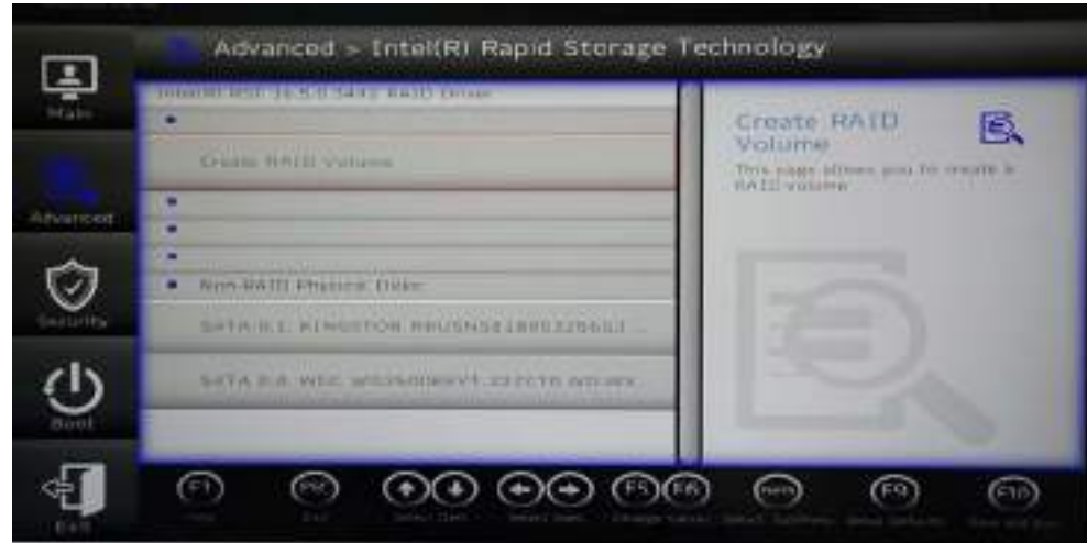
Figure 6 - 1 Create RAID Volume
